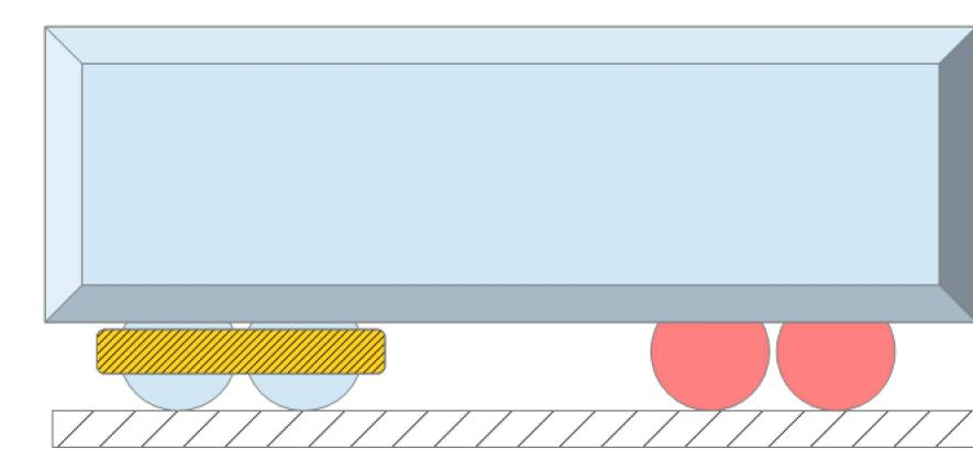
1007 retrofit added Rail generator using the rotation of rail wheels to generate current to store on railway car Copyright © Christopher g Brown 2017
